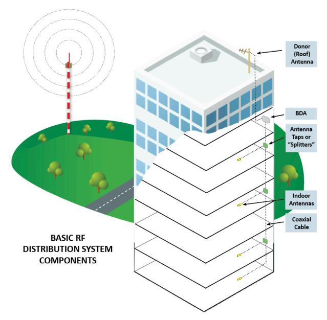
1. Donor (roof) antenna. This is called the "DONOR" antenna. It is usually mounted on the roof, or
