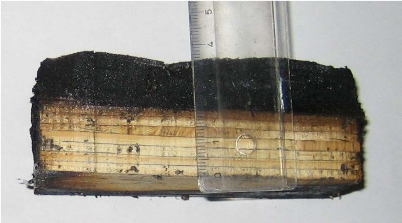
FIGURE 1: INTUMESCENT CHAR COATING ON LAMINATE VENEER LUMBER (TAKEN FROM: HAKKARAINEN, 2010) 4
